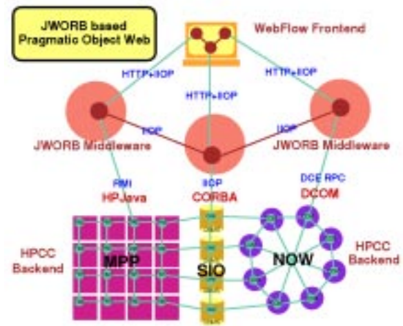
Figure 8: Overall architecture of the JWORB based Pragmatic Object Web middleware
