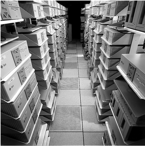
Figure 4: 100-Node 200-CPU Cluster Key points: no people, no monitors, no visible cables, extreme symmetry, internal disks.
