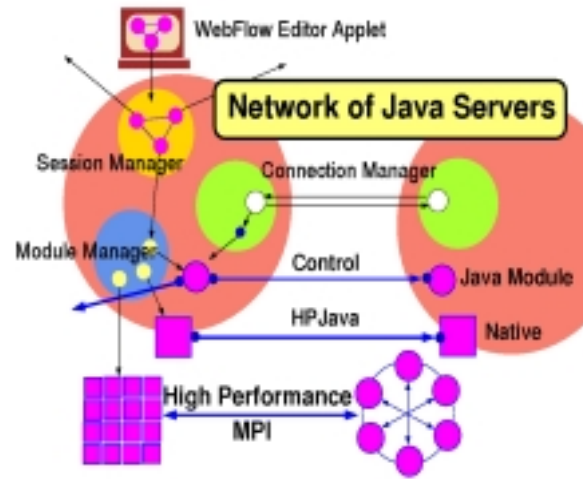
Figure 19: Overall Architecture of the 3-tier WebFlow model with the visual editor applet in tier-1, a mesh of Java Web Servers in tier 2 (including WebFlow Session Manager, Module Manager and Connection Manager servlets), and (high performance) computational modules in tier-3.
