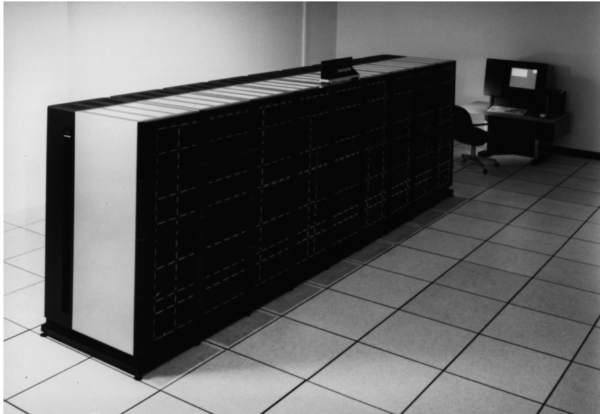
Figure 8: The “Delta Touchstone” Parallel Supercomputer Installed at Caltech and Produced by Intel
