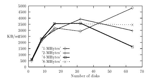
Figure 3: Read Rates for Single Compute Node-Burst Mode
