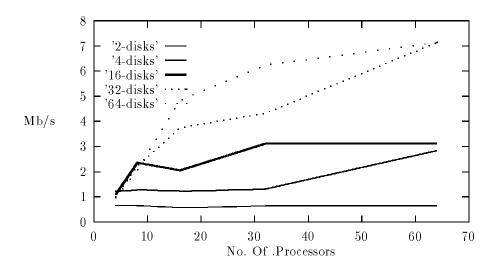
Figure 9: Multicompute Nodes Read (Mode 2 and 16 Mbytes File )
