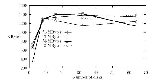
Figure 4: Write Rates for Single Compute Node-Burst Mode
