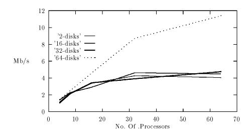
Figure 5: Read Rates For Multiple Compute Nodes - Mode 0
