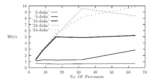
Figure 8: Multicompute Nodes Read (Mode 3 and 16 Mbytes File)
