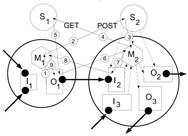
**Figure 1** This diagram illustrates point-to-point communication between Web servers, used to implement a webflow channel between compute-web modules. Two extreme implementation modes are described: a) based on today's Web server technology, and b) based on thread memory mapped high performance implementation, expected in future Web compute-servers. Subsequent steps, represented by a sequence of labelled lines in the figure, are described below in both implementation modes.
