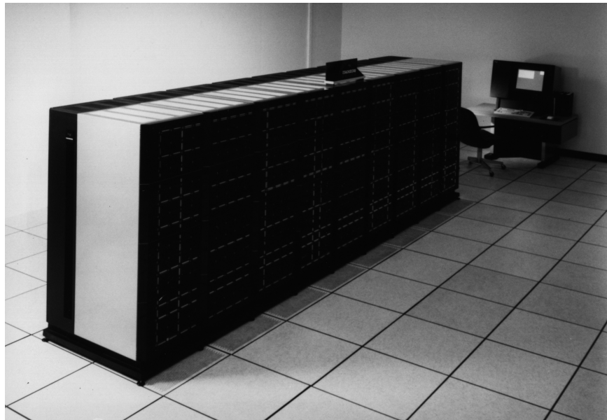
Figure 8: The “Delta Touchstone” Parallel Supercomputer Installed at Caltech and Produced by Intel. This system uses a mesh architecture linking 512 nodes, and was a prototype for the Paragon.
