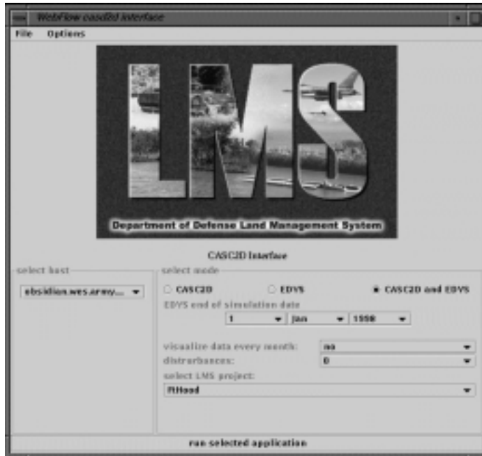
Fig. 21: LMS front-end simulation panel. The controls allow for selecting the simulation mode: Casc2d alone, Edys alone, and both simulations coupled, as described in Section 4.3. In the latter case, the user also provides the end date of the Edys run, Edys visualization toggle and disturbances, the directory that contains casc2d input data files and finally the user select the host on which the casc2d simulation is to be run.
