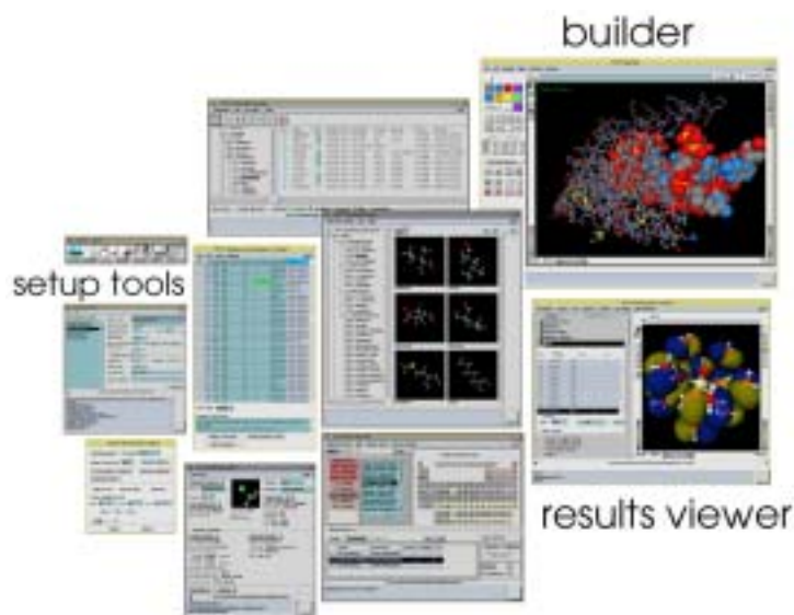
Figure 3. A collage of Ecce tools showing setup tools such as an editor, basis set tool and builder, a job submission tool, a results viewer, and a tool to manage calculations.
