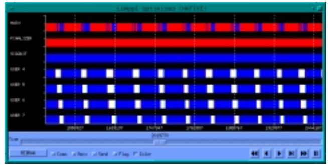
Figure 10: Visualization of the LUAppl running with the Java Threads transformation (4 threads) and the pthread_setconcurrency service
