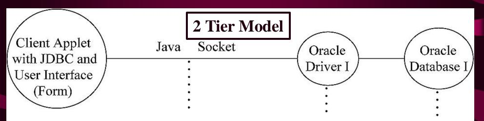
In this model, linking to database servers can be established as many Java Socket connections. Each connection will link to a driver and a database server, but Oracle database servers can talk to each other via SQL\*Net.
