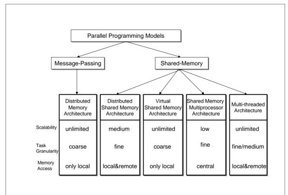
Figure 4 1. Message-passing and shared-memory programming models implemented on top of various types of parallel architectures, and their prominent features.
