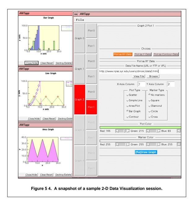
Currently the system supports line and scatter plots, bar charts, area graphs, and contour graphs. The graphs can be annotated with a title and axis labels in various font styles and colors. Users can view multiple data sets within the same window, the same data set in different windows, or different data sets in different windows.
