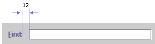
FIGURE 135 Spacing Between A Label and a Component
