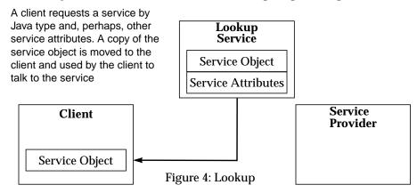
A client locates an appropriate service by its type—that is, by its interface written in the Java programming language—along with descriptive attributes which are used in a user interface for the lookup service. The service object is loaded into the client.
