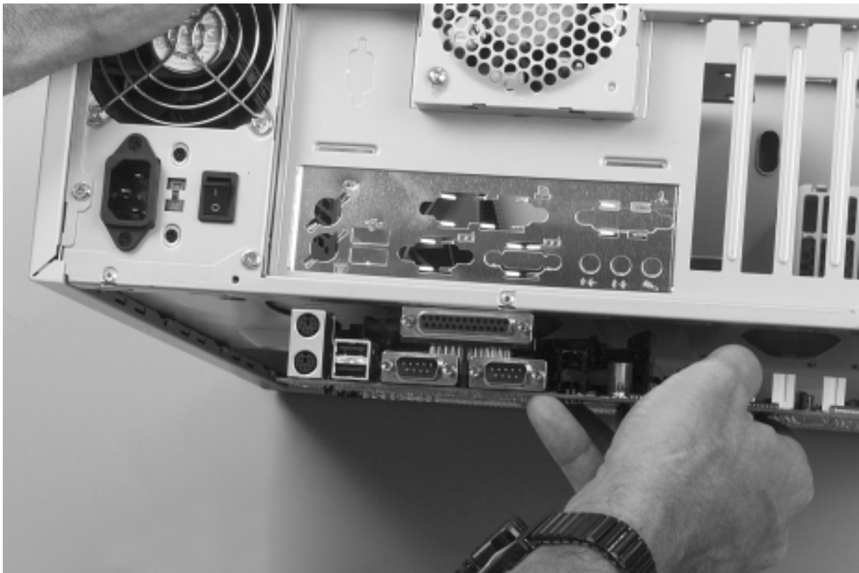
Photo 21. Locate the Punchout Access Ports
