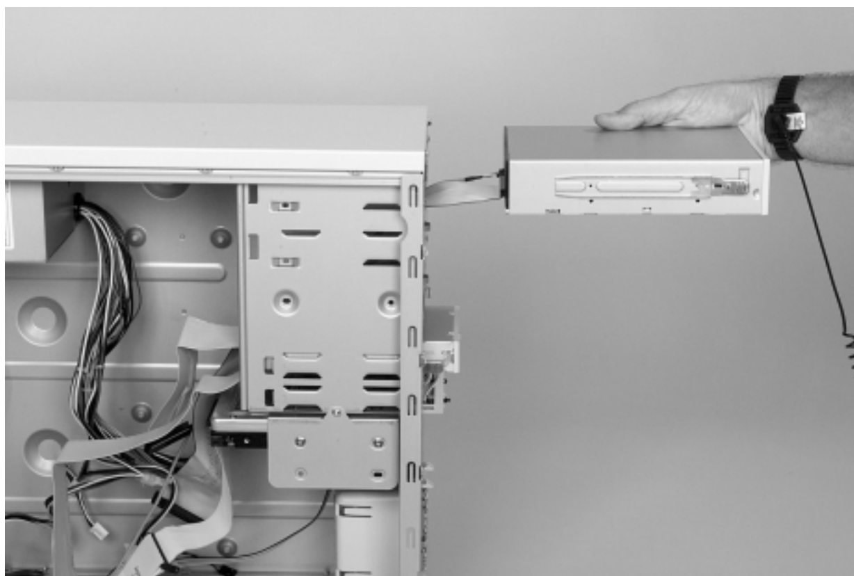
Photo 13. The Drives Installed in the Case
