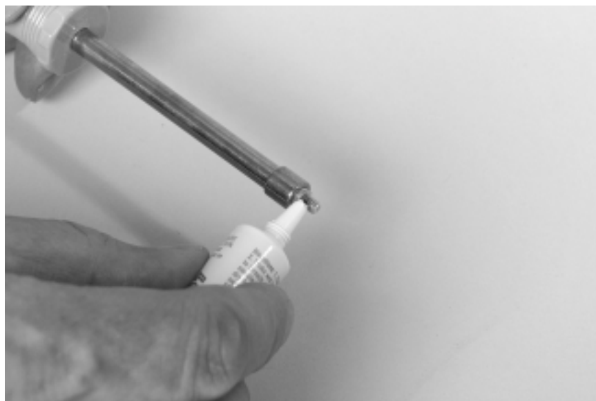
Photo 24. Placing Loctite on the Male Threads of the Extra Standoff
