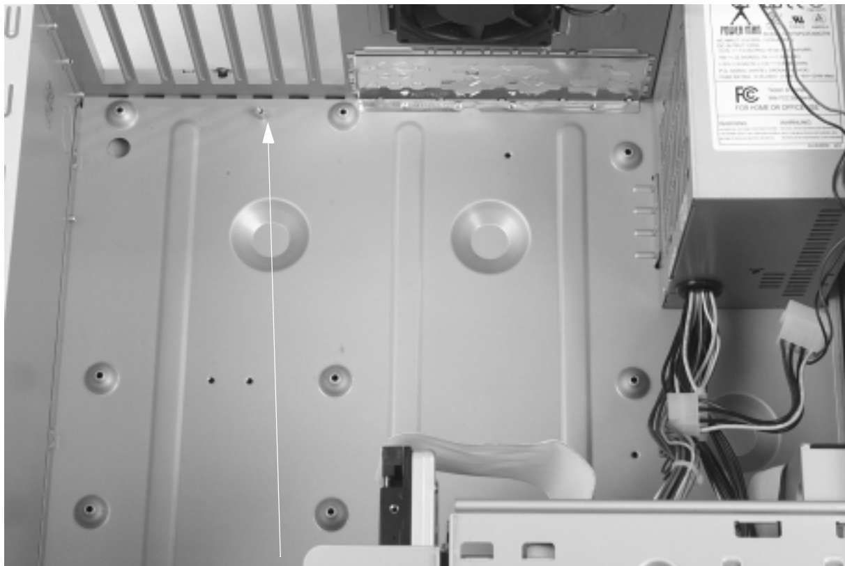
Photo 26. An Extra Standoff That has been Installed
