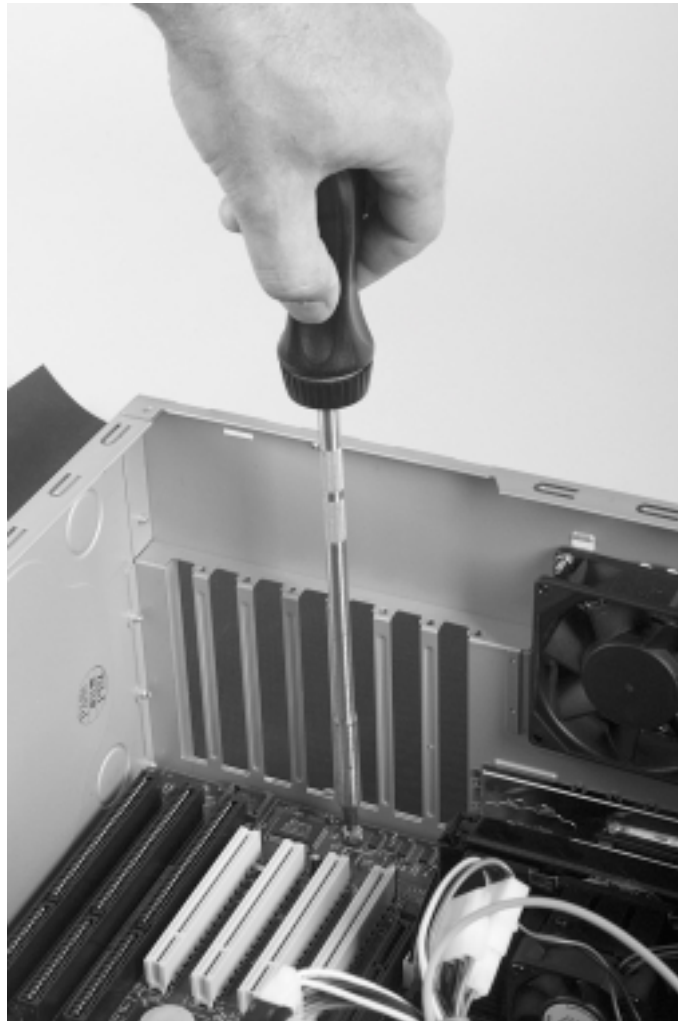
Photo 36. Install Motherboard on Standoffs and Tighten Screws
