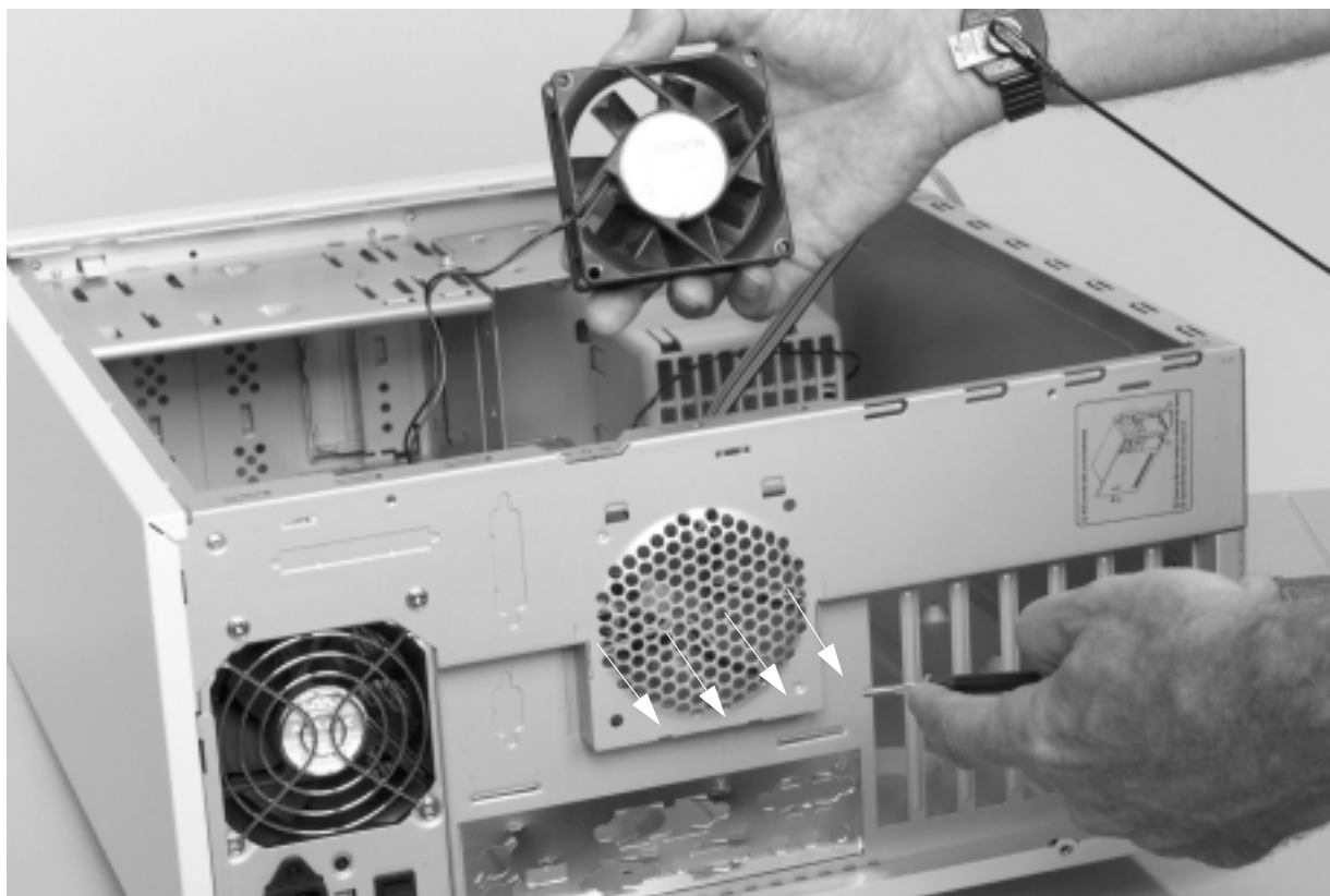
Photo 6. An Exhaust Fan in the Rear of the Case
