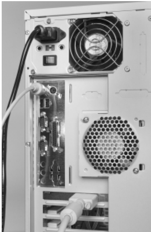
Photo 50. Power Cable Installed
