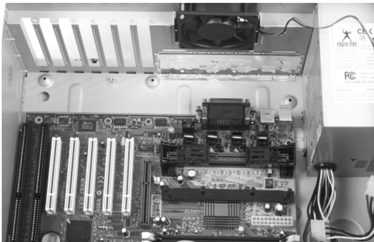
Photo 27. Check Alignment of the Motherboard with Standoff Holes
