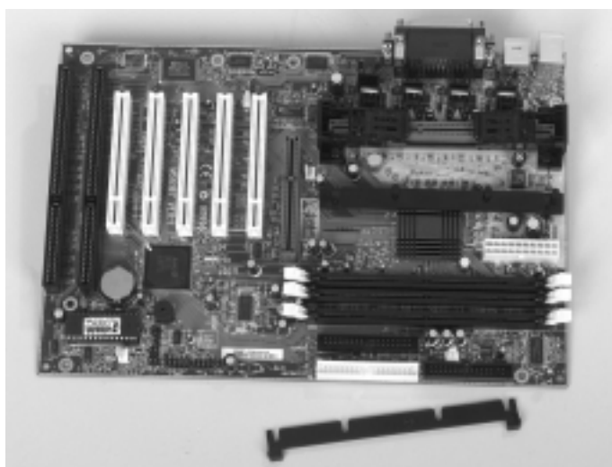
Photo 18. Top of Motherboard, Installing the Heatsink Support
