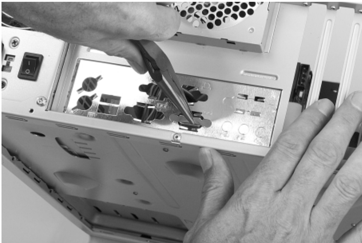
Photo 22. Removing an Access Port
