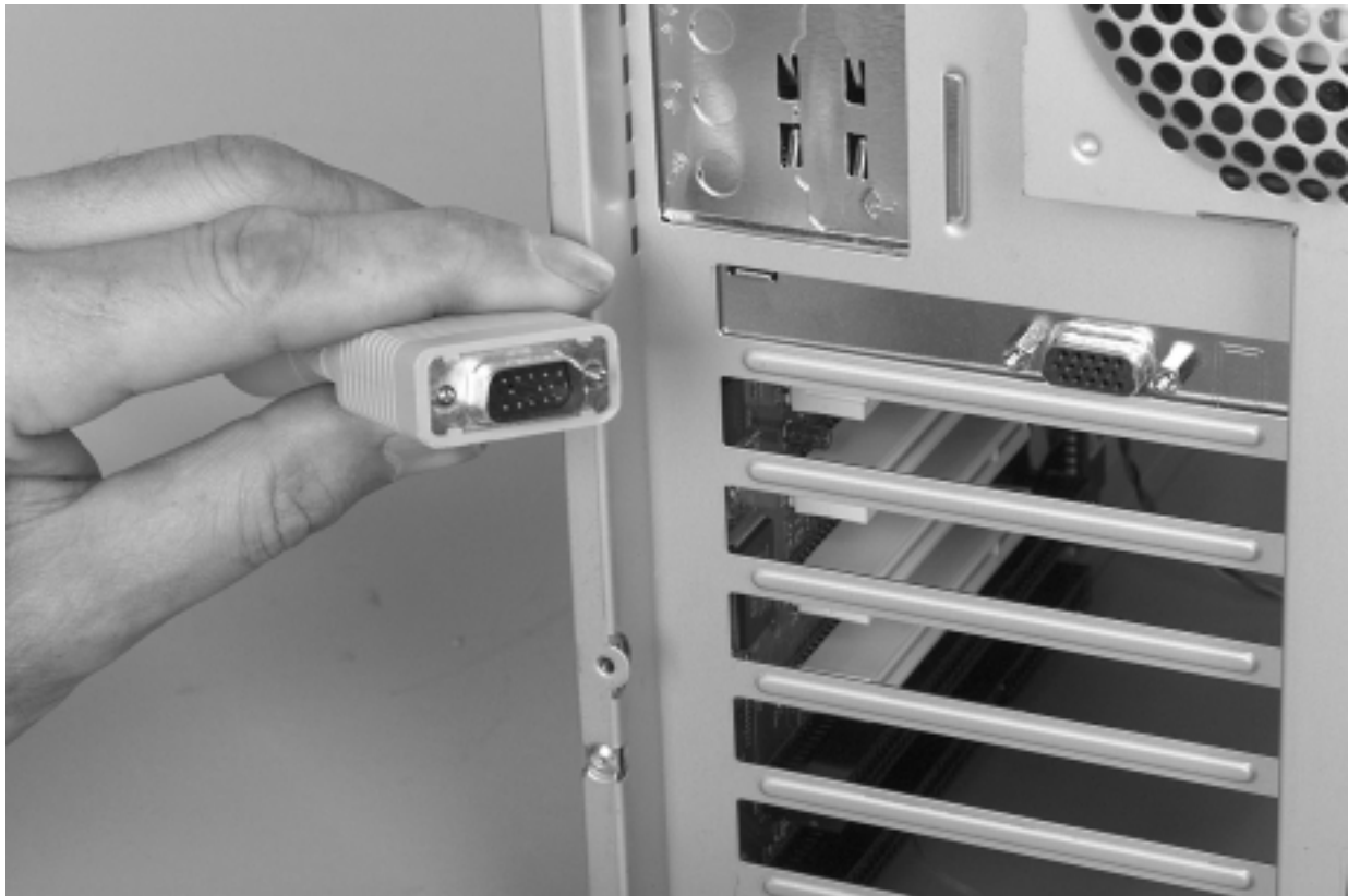
Photo 48. Install Monitor Cable
