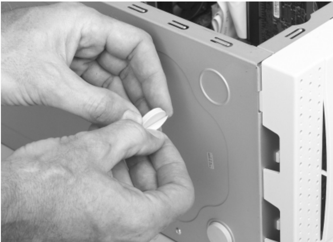
Photo 46. Install Feet on Enclosure
