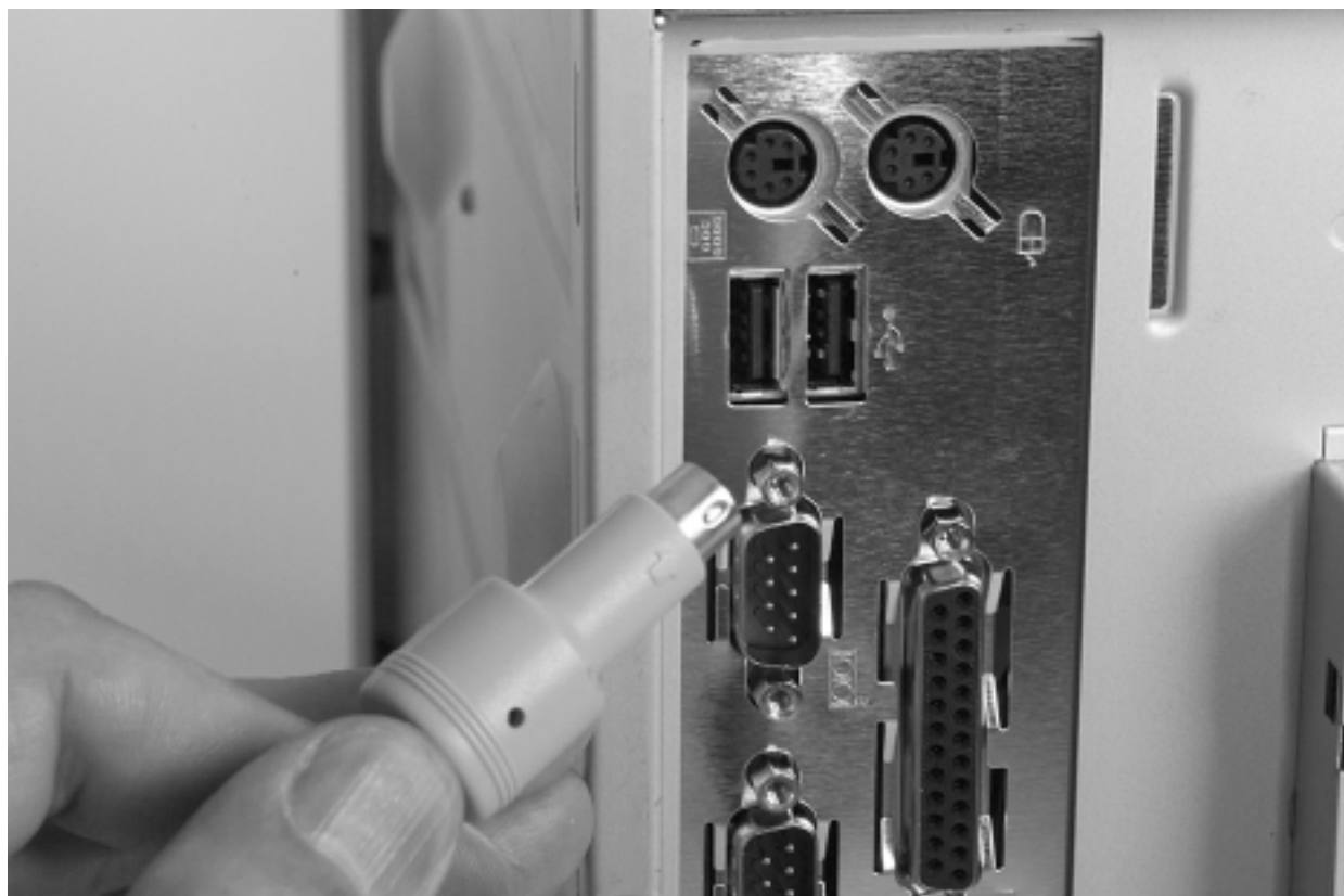
Photo 47. Keyboard and Mouse Cable Connectors
