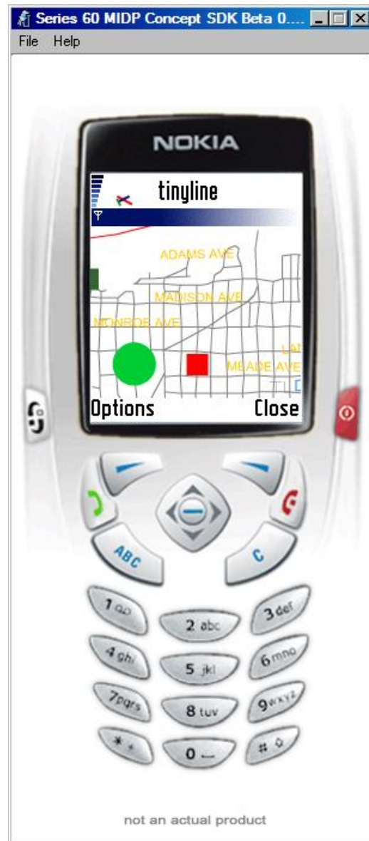
Figure 6. An SVG document fragment for a portion of San Diego displayed in TinyLine SVG viewer.
