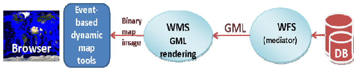
Figure 2: The ordinary system test set-up. Any-data is converted to common structured data (GML) and rendered as map images.
